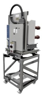
The **SG40** maintains the reliable, field-proven design of the MILE family, suited for higher voltage ratings of up to 36 kV. Its typified design ensures that the arrangement of equipment and instruments in the panel reflects the common switchgear configuration preferred by customers globally. The floor truck design facilitates the easy removal and maintenance of the vacuum circuit breaker, ensuring efficient servicing.
